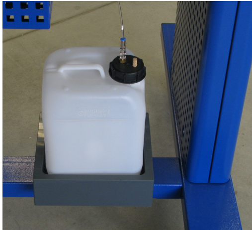
Fig. 3.12 Fuel tank - fuel solenoid valve and pump are located under the table
